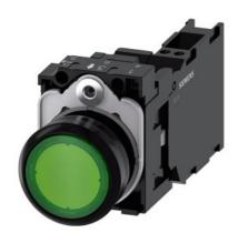
Illuminated pushbutton, 22 mm, round, plastic, green, pushbutton, flat, momentary contact type, with holder, 1 NO+1 NC, LED module with integrated LED 110 V AC, spring-type terminal, with laser labeling, symbol number according to, ISO 7000 or IEC 60417
