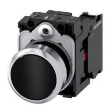
Pushbutton, 22 mm, round, metal, shiny, black, pushbutton, flat, momentary contact type, with holder, 1 NC, screw terminal, with laser labeling, upper case and lower case, always upper case at beginning of line
