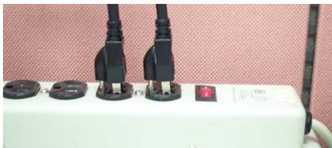
Figure 3.10: Power cord plugs should have same orientation in the socket/ 插座上电源线方向相同 / 插座上的电源线方向應相同
