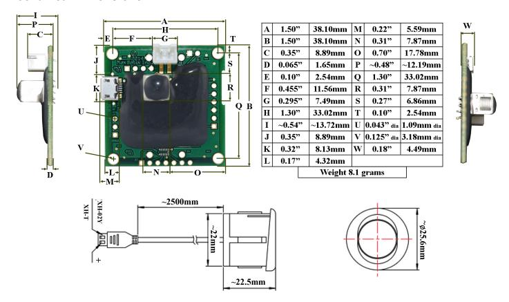
The recommended operating and storage temperature of the MB8450 USB-CarSonar-WR is -40C to +75C.
