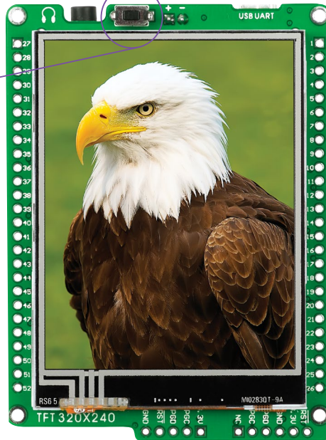
Figure 4-2: Frontal reset button
