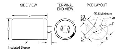
DescriptionSnap-In, Aluminum ElectrolyticRoHSYesLead3 Pin ShortAEC-Q200NoComponent Weight64 gNotesAdd 0.5mm To D And 1mm To L For Sleeving.Shelf Life208 Weeks
