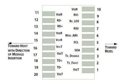
Pin-out of connector Block on Host board
