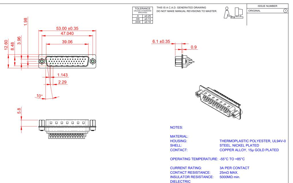
WITHSTANDING VOLTAGE: 1000V AC rms
