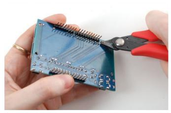
Finish up by carefully clipping the leads. For some Arduinos, the long leads may interfere with headers or parts on the Arduino board so we suggest just clipping them all. Do it carefully as these are a little difficult to cut and may fly at you. We suggest doing it over a trash can.
