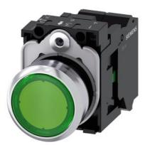
Illuminated pushbutton, 22 mm, round, metal, shiny, green, pushbutton, flat, momentary contact type, with holder, 1NO, LED module with integrated LED 110 V AC, spring-type terminal, with laser labeling, symbol number according to, ISO 7000 or IEC 60417
