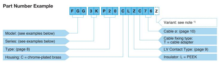
FGG.3K.P20.CLZC76Z = Straight plug with key (G), 3K series, multi fluid with 2 times P1 contacts, chrome-plated brass housing, PEEK insulator, C type collet for 7.5 mm diameter cable, and nut for fitting a bend relief.
