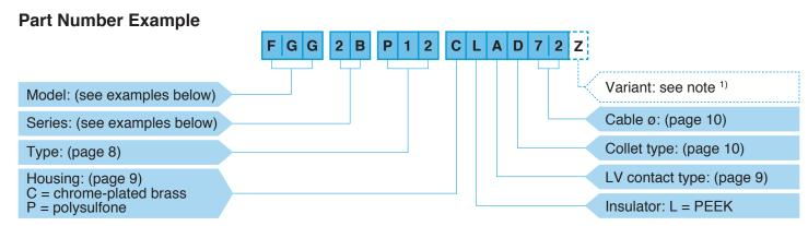
**FGG.2B.P12.CLAD72Z** = Straight plug with key (G), 2B series, mixed type to accept one P1 fluid contact and 4 low voltage electrical contacts, chrome-plated brass housing, PEEK insulator, 4 male solder electrical contacts, type D collet system to suit a 6.1 to 7.0 mm diameter cable, and a nut for fitting a bend relief.
