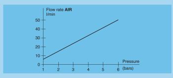
Note: test carried out with a 2 mm inner diameter tube.
