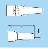
A bend relief made from thermoplastic polyurethane elastomer can be fitted over LEMO plugs and sockets that are supplied with nut for fitting such bend relief.
