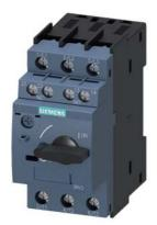
Circuit breaker size S0 for motor protection, CLASS 10 A-release 23...28 A N-release 364 A screw terminal Standard switching capacity with transverse auxiliary switches 1 NO+1 NC
