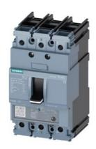
circuit breaker 3VA5 UL frame 125 breaking capacity class H 65kA @ 480 V 3-pole, line protection TM230, FTAM, In=100A overload protection Ir=100A fixed short-circuit protection Ii=5...10 x In UL489 SB (naval), 50 deg. cel. cable connection on both sides
