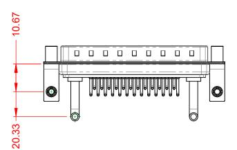
OPERATING TEMPERATURE:-55°C ~ 125°CPOWER/CO-AX CONTACT RATING:30A (CURRENT)(IF PRESENT)SIGNAL CONTACT CURRENT RATING:5A PER CONTACTSIGNAL CONTACT RESISTANCE:10mΩ MAX.INSULATOR RESISTANCE:5000MΩ min.DIELECTRIC2000MΩ min.
