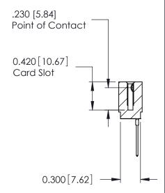
ACAD REFERENCE NO. 725-ENG MASTER 725 Series Ultra-Mate Card Edge Connector - Press Fit SEGAHOM:3A:9A DRAWN: J.LEE Part Number: 725-007-545-101 CHECKED: DATE: **EDAC INC** SCALE: SHEET 1 OF 1 THESE DRAWINGS AND SPECIFICATIONS ARE THE PROPERTY OF EDAC INC.,AND TORONTO, ONTARIO SHALL NOT BE REPRODUCED, OR COPIED DRAWING NUMBER **ISSUE** CANADA OR USED AS THE BASIS FOR THE 725-ENG MASTER MANUFACTURE OR SALE OF APPARATUS YOUR CONNECTION TO QUALITY & SERVICE WITHOUT WRITTEN PERMISSION.
