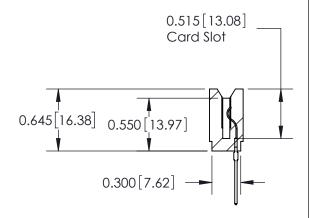
737 Series Ultra-Mate Card Edge Connector - Press Fit Part Number: 737-016-540-106 **EDAC INC** THESE DRAWINGS AND SPECIFICATIONS
