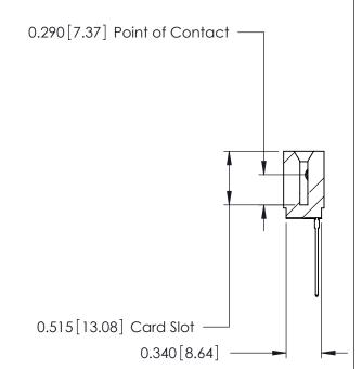
ACAD REFERENCE NO. 746-ENG MASTER 746 Series Ultra-Mate Card Edge Connector - Press Fit DRAWN: J.LEE DATE: AUG 20/09 Part Number: 746-015-541-101 CHECKED: DATE: **EDAC INC** SCALE: SHEET 1 OF 1 THESE DRAWINGS AND SPECIFICATIONS ARE THE PROPERTY OF EDAC INC.,AND TORONTO, ONTARIO SHALL NOT BE REPRODUCED, OR COPIED DRAWING NUMBER **ISSUE** CANADA OR USED AS THE BASIS FOR THE 746-ENG MASTER MANUFACTURE OR SALE OF APPARATUS YOUR CONNECTION TO QUALITY & SERVICE WITHOUT WRITTEN PERMISSION.
