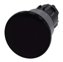
Mushroom pushbutton, 22 mm, round, plastic with metal front ring, black, 40 mm, latching, pull-to-unlatch mechanism, Z=50-unit packaging
