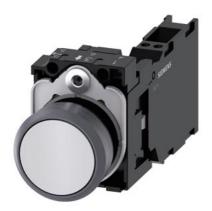
Pushbutton, 22 mm, round, plastic with metal front ring, white, pushbutton, flat, momentary contact type, with holder, 1 NO+1 NC, spring-type terminal, with laser labeling, symbol number according to, ISO 7000 or IEC 60417
