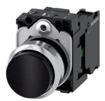
Pushbutton, 22 mm, round, metal, shiny, black, pushbutton, raised, momentary contact type, with holder, 1 NO, screw terminal, with laser labeling, upper case and lower case, always upper case at beginning of line
