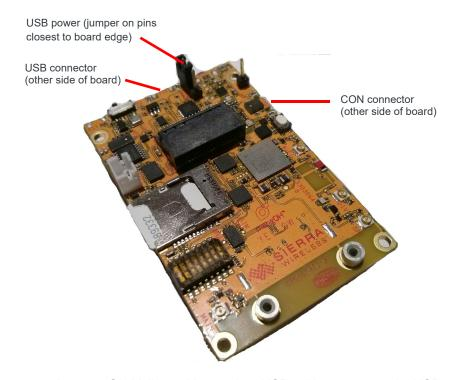
3. Power up the mangOH Yellow—Use a micro-USB cable to connect the USB connector to a powered USB port on your computer.
