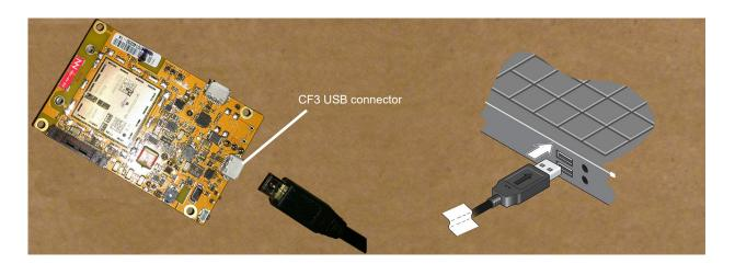
**Important:** If LTE-M coverage is not available, the mangOH Yellow's WP7702 module will fall back to 2G, which consumes up to 2 A of current for short bursts. In this case, USB power is insufficient (500 mA) and the module may repeatedly brown out and reboot. Use a Li-ion or Li-polymer (3.7 V nominal) battery to supply sufficient power. (See the mangOH Yellow User Guide for details.)
