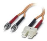
Assembled FO cable, zip cord cable, multi-mode fiberglass 50/125  $\mu$ m, OM2, plug: SC duplex/B-FOC (ST), degree of protection: IP20, for installation in cable ducts or control cabinets, length: 1 m
