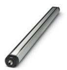
LED machine light, 24 V DC, emission angle 75 °/95 °, color temperature 5000 K, length 1070 mm, diameter 70 mm, M12 connector, Light housing: Anodized aluminum, Pane: Single-pane safety glass (ESG, thermally toughened float glass), pivoting, resistant to coolants and lubricants
