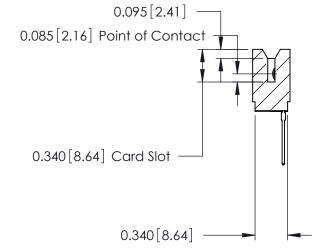
ACAD REFERENCE NO. 746 Series Ultra-Mate Card Edge Connector - Press Fit DRAWN: J.LEE Part Number: 746-026-540-506 CHECKED: **EDAC INC** SCALE: THESE DRAWINGS AND SPECIFICATIONS ARE THE PROPERTY OF EDAC INC., AND TORONTO, ONTARIO SHALL NOT BE REPRODUCED, OR COPIED DRAWING NUMBER CANADA OR USED AS THE BASIS FOR THE 746-ENG MASTER MANUFACTURE OR SALE OF APPARATUS YOUR CONNECTION TO QUALITY & SERVICE WITHOUT WRITTEN PERMISSION.
