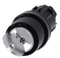
RONIS key-operated switch, 22 mm, round, plastic, lock number 455, with 2 keys, 2 switch positions O-I, latching, actuating angle 90°, 10:30h/13:30h, key removal O, with laser labeling, upper case and lower case, always upper case at the beginning of the word
