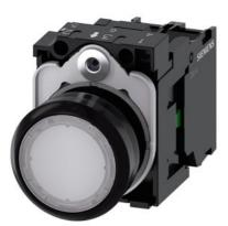
Illuminated pushbutton, 22 mm, round, plastic, white, pushbutton, flat, momentary contact type, with holder, 1NO, LED module with integrated LED 230 V AC, screw terminal, with laser labeling, upper case and lower case, Always upper case at the beginning of the word
