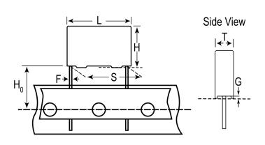
Dielectric Metallized Polypropylene Style Radial Features MKP EMI Safety RoHS Lead Wire Leads Safety Class X2 Qualifications ENEC, UL, cUL, CQC AEC-Q200 No THB Performance No 1.057 g Component Weight Miscellaneous ClimCat: 40/110/56/B Shelf Life 104 Weeks
