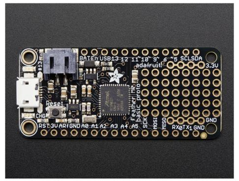
At the Feather M0's heart is an ATSAMD21G18 ARM Cortex M0 processor, clocked at 48 MHz and at 3.3V logic, the same one used in the new Arduino Zero (http://adafru.it/2843). This chip has a whopping 256K of FLASH (8x more than the Atmega328 or 32u4) and 32K of RAM (16x as much)! This chip comes with built in USB so it has USB-to-Serial program & debug capability built in with no need for an FTDI-like chip.
