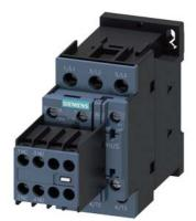
power contactor, AC-3 17 A, 7.5 kW / 400 V 2 NO + 2 NC, 42 V AC, 50 Hz, 3-pole, Size S0 screw terminal Removable auxiliary switch
