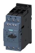
Special type Circuit breaker size S2 for motor protection, CLASS 10 Arelease 22...32 A N-release 416 A screw terminal Standard switching capacity with transverse auxiliary switches 1 NO+1 NC Ambient temperature -50 °C 250 switching cycles
