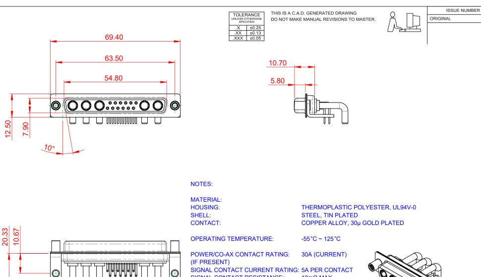
SIGNAL CONTACT CURRENT RATING: 5A PER CONTACT SIGNAL CONTACT RESISTANCE:  $10m\Omega$  MAX.
