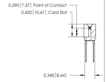
726 Series Ultra-Mate Card Edge Connector - Press Fit Part Number: 726-052-553-201 **EDAC INC** THESE DRAWINGS AND SPECIFICATIONS
