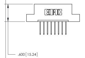
INSULATOR MATERIAL: THERMOPLASTIC POLYESTER, UL 94V-0 CONTACT MATERIAL; COPPER, NICKEL, TIN ALLOY CA-725
