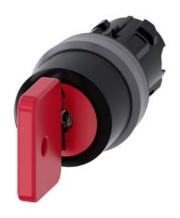
Key-operated switch O.M.R, 22 mm, round, plastic with metal front ring, lock number 73037, red, with 2 keys, 3 switch positions I-O-II, latching, actuating angle  $2x45^{\circ}$ , 10:30h/12h/13:30h, key removal O+I, with laser labeling, lower case
