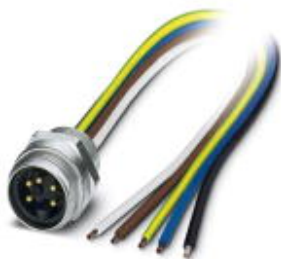
Sensor/actuator flush-type plug, 5-pos., 7/8", front mounting with Pg13.5 thread, with 0.5 m PVC litz wire, 5 x 0.75 mm 2
