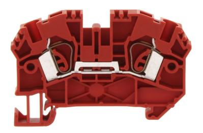
Feed-through terminal, Tension-spring connection, Mounting type: Mounting rail TS 35/7.5, Rated cross-section: 4 mm², Width: 6.1 mm, Colour: Red
