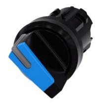
Selector switch, illuminable, 22 mm, round, plastic, blue, selector switch, short, 2 switch positions O<I, momentary contact type, Actuating angle 45°, 10:30h/12h, with laser labeling, lower case
