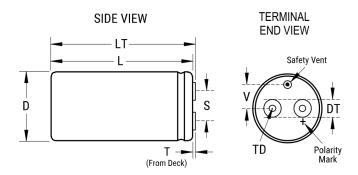
General Information Series ALS30 Dielectric Aluminum Electrolytic Description Screw Terminal, Aluminum Electrolytic RoHS AEC-Q200 No Component 1450 g Weight Dimensions D And L Include Sleeving. MS (MxH) = Notes M12x16. Mounting Clamp (Sold Separately): V11 Shelf Life 156 Weeks
