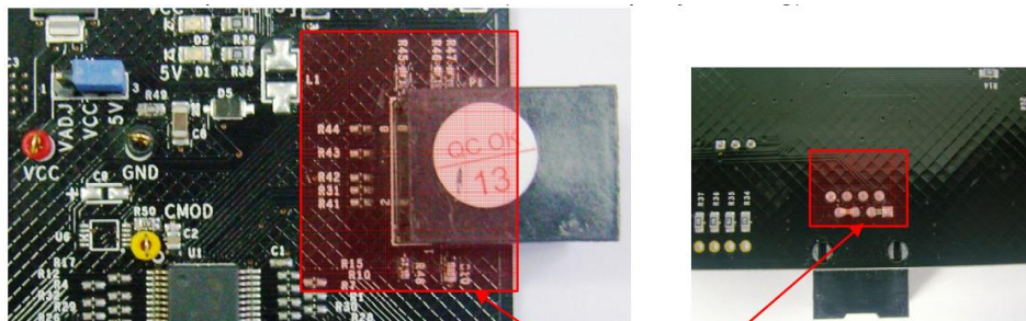
Figure 2. Board Reworded with OCD Termination
