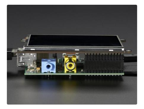
Uses the hardware SPI pins (SCK, MOSI, MISO, CE0, CE1) as well as GPIO #25 and #24. GPIO #18 can be used to PWM dim the backlight if you like. All other GPIO are unused. There's a 2x13 header on the bottom, you can connect a standard Pi GPIO cable to it to use any of the other pins ask you like
