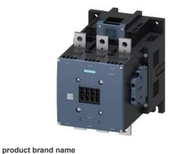
power contactor, AC-3 500 A, 250 kW / 400 V AC (50-60 Hz) / DC 110-127 V AC/DC auxiliary contacts 2 NO + 2 NC 3-pole, frame size S12 busbar connections drive: conventional screw terminal NEMA version
