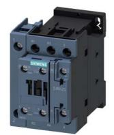
Power contactor, AC-3 25 A, 11 kW / 400 V 2 NO + 2 NC 220 V AC, 50 Hz 240 V, 60 Hz 4-pole Size S0 Screw terminal 1 NO + 1 NC integrated
