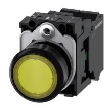
Illuminated pushbutton, 22 mm, round, plastic, yellow, pushbutton, flat, momentary contact type, with holder, 1NO, LED module with integrated LED 24 V AC/DC, spring-type terminal, with laser labeling, inscription or symbol Customer-specific selection with SIRIUS ACT configurator (CIN)
