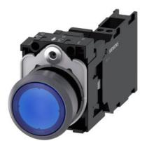
Illuminated pushbutton, 22 mm, round, plastic with metal front ring, blue, pushbutton, flat, momentary contact type, with holder, 1 NO+1 NC, LED module with integrated LED 24 V AC/DC, spring-type terminal, with laser labeling, upper case and lower case, Always upper case at the beginning of the word
