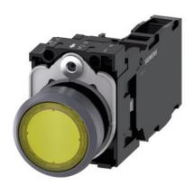
Illuminated pushbutton, 22 mm, round, plastic with metal front ring, yellow, pushbutton, flat, momentary contact type, with holder, 1 NO+1 NC, LED module with integrated LED 110 V AC, screw terminal, with laser labeling, upper case and lower case, always upper case at beginning of line
