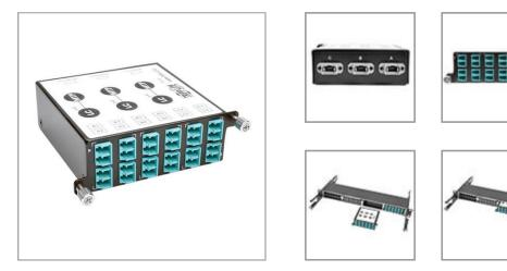
Installs in select Tripp Lite fiber chassis to connect 12 duplex LC fiber cables with three 8-fiber MTP/MPO connections in high-density network applications.
