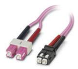
Assembled FO cable, zip cord cable, multi-mode fiberglass 50/125  $\mu$ m, OM4, plug: SC duplex/SC-RJ, degree of protection: IP20, for installation in cable ducts or control cabinets, length: 2 m
