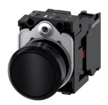
Pushbutton, 22 mm, round, plastic, black, pushbutton, flat, momentary contact type, with holder 1 NC, screw terminal, with laser labeling, symbol number according to, ISO 7000 or IEC 60417
