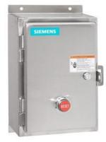
Non-reversing motor starter, Size 1, Single phase full voltage, Solid-state overload relay, OLR amp range 5.5-22A, 110V 50Hz / 120V 60Hz coil, Non-combination type, Encl. type 4X 304 S. Steel, Water/dust tight noncorrosive, Standard width enclosure
