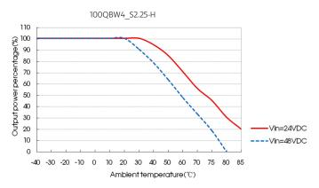
Note: Temperature Derating Curves were tested at natural convection (20FLM).
