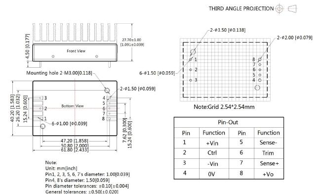
Mounting hole screwing torque: Max 0.4 N·m
